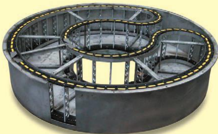
Application with 2 chains. Rotation 370°
