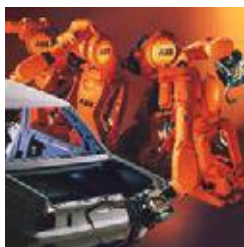
Circular nylon chains on welding robots.
