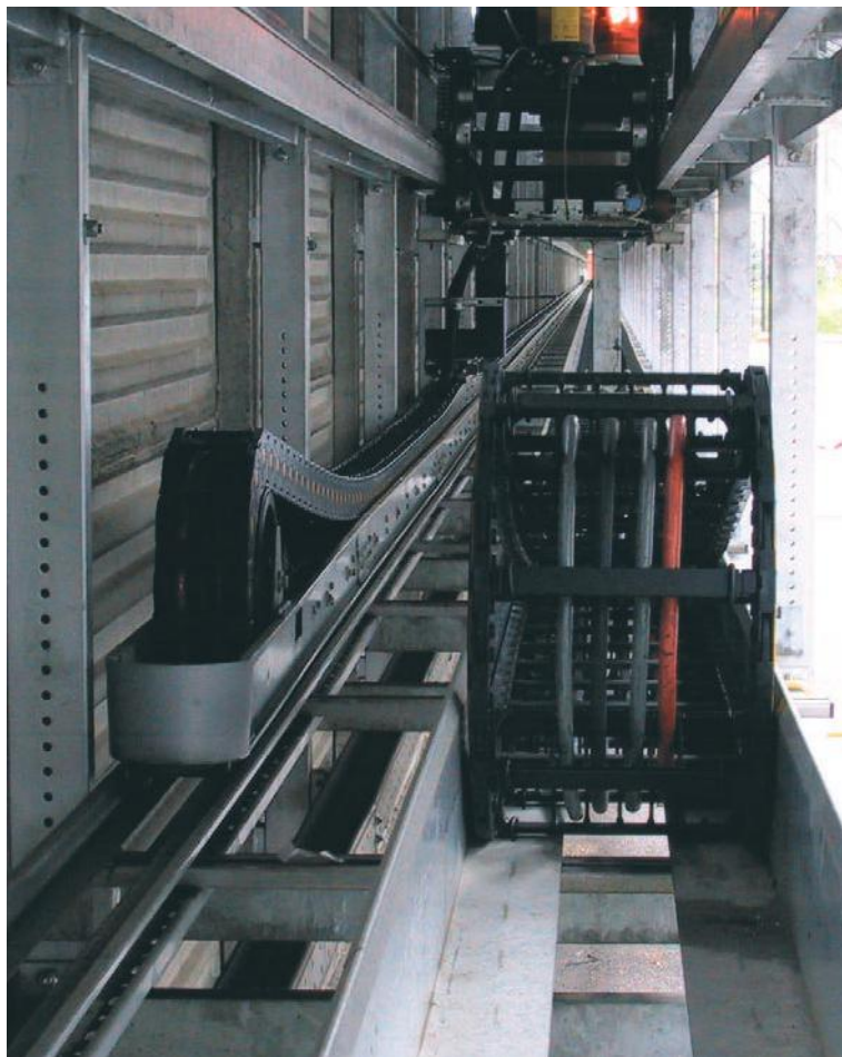
Chain testing rig for long travel: Tests at 8 m/s for 130 m travels.
