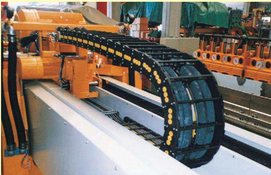
Nylon chain, type 310, in a self-supporting state.
